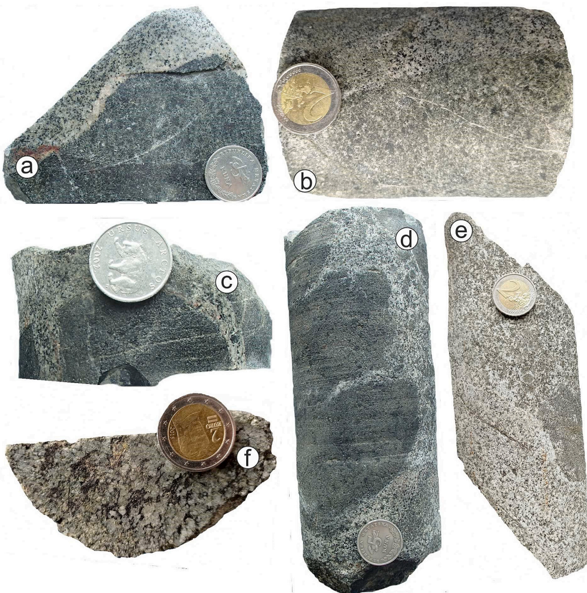
Fig. 5. Samples from Drava Depression: a) sharp contact between monzogranite-granodiorite and microgranular mafic enclave (MME), characterized by leucocratic halo; b) contact between monzogranite-granodiorite and intermediate rock (IMR); c) angular MME in monzogranite-granodiorite (D-1-19-4-9); d) larger pillow-like MME (D-1-9G) and numerous smaller MME in monzogranite-granodiorite (D-1-9G); e) disaggregated MME in monzogranite-granodiorite (D-1-17-7-35); the composition of the area where MME is disaggregated fully resembles composition of the IMR; f) gneiss (D-1-22G).
