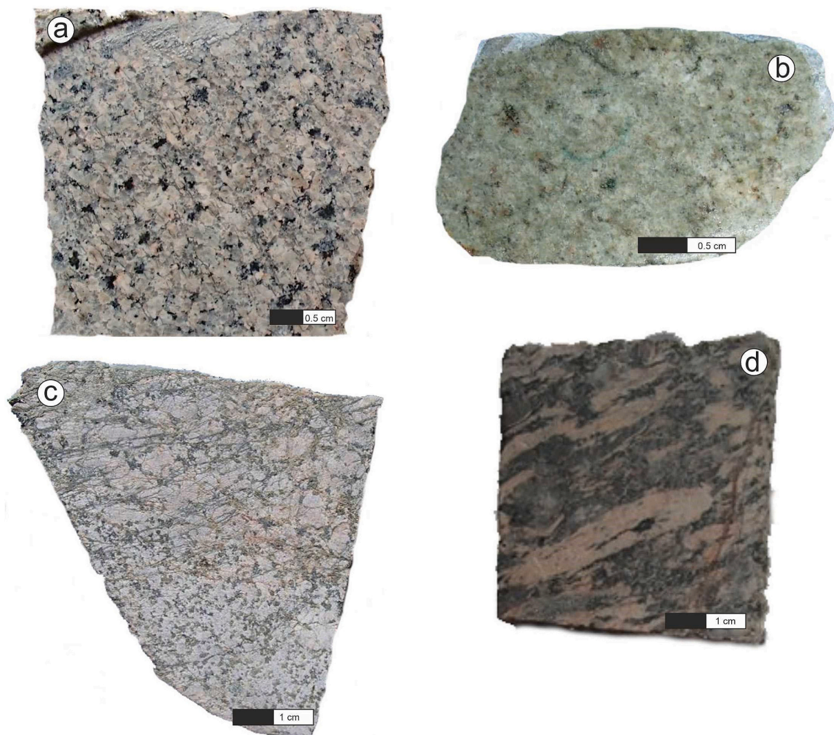
Fig. 4. Samples from Slavonija-Srijem Depression: a) alkali-feldspar granite (B-1-5), b) alkali-feldspar granite (B-2-1), c) quartz-alkali-feldspar syenite (B-3-5); d) orthogneiss (B-5-2).
